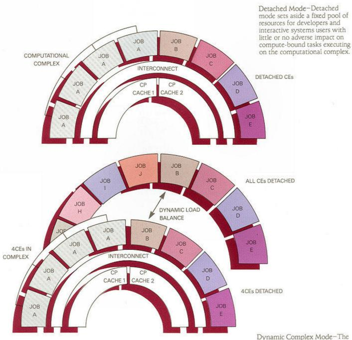
computational complex mode—frie computational complex can be time- and load-multiplexed between two modes: all CEs in the complex attached and all detached. This assures maximum throughput for a varying mix of production and development jobs.
