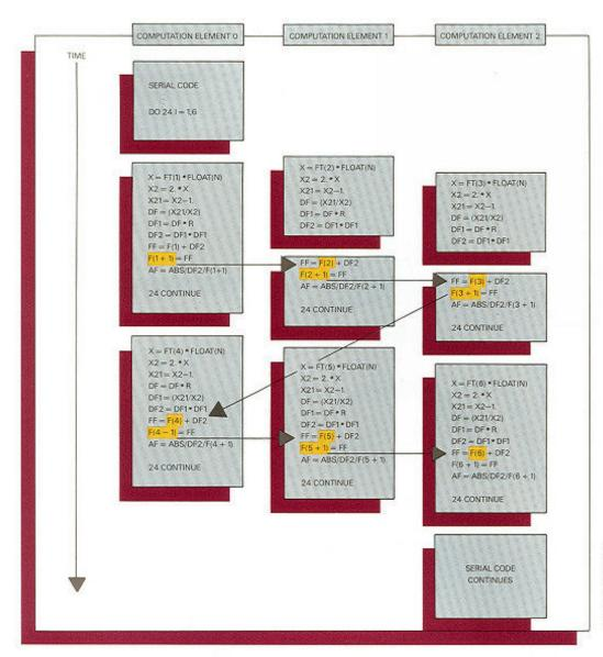
Loops with intra-loop data dependencies that automatically optimize for parallel execution, would run in scalar mode on traditional scalar or vector-only architectures.
