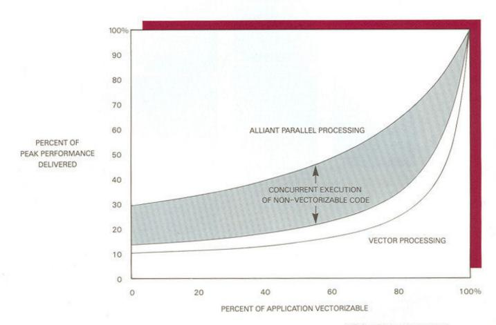
With Alliant concurrency, FX/Fortran can optimize more of an application, delivering more of the computer's peak performance than would be possible with vector-only processors. Compared with vector computers, the FX/8 provides greater absolute performance and faster time-to-solution.
