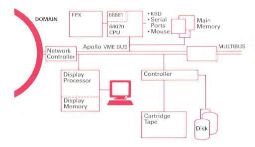
The DN570's Integrated Architecture. The DN570 features a modular architecture that integrates high-performance graphics into the computing environment. The Graphics/Processor, Mass Storage, and MULTIBUS modules communicate at bus speeds with each other and with the DOMAIN System network. This total integration provides the highest levels of functionality and performance.
