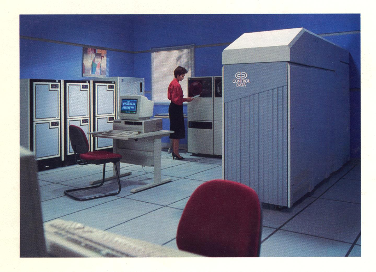
Mid-range, generalpurpose mainframes, the air-cooled CYBER 960 models utilize the most advanced ECL chip technology available.
