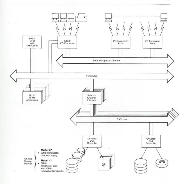
The Universe 68 is organized around three bus structures. The primary system bus is the 32-bit VERSAbus, which provides a bandwidth of up to 20M bytes/second. The VERSAbus interfaces the main 68000 processor, main memory, and channel control processors. One or more selector channel interface subsystems can be used to interface burst mode or block transfer devices. Devices on the selector channel
