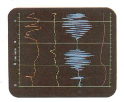
A combination of split screen, user defined characters, cursor addressing and smooth scroll can be used to create continuous chart recorder effects for monitoring scientific data.
