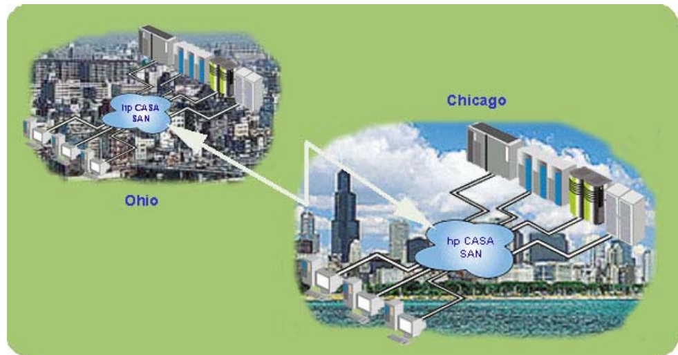
figure 6. The CASA allows data to be mirrored synchronously or asynchronously between geographically remote locations using an IP-based network.
