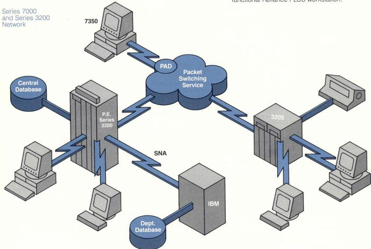
The OS/32 communications package is configurable for both local and remote (modem) operating environments. Using Series 3200 machines as gateways, the operator can use terminal emulation to access the PENnet Plus network. This gives access to systems connected locally via Ethernet (IEEE 802.3) or remotely via the X.25 packet switching services.
