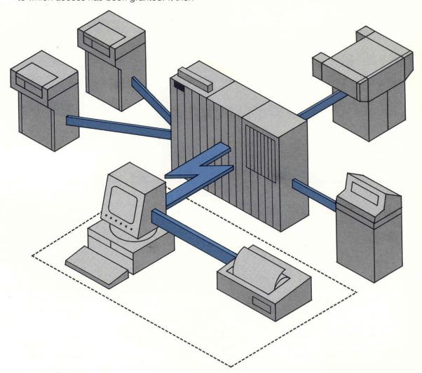
For connection to OS/32 based Series 3200 machines, an optional package is available providing both file transfer and PE 6300 terminal emulation.
