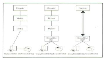
S/370 data channel. In all cases the equipment is compatible with the IBM 3270.
