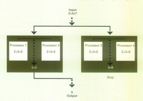
Stratus systems are designed to survive component failure without any performance degradation. Self-checking logic detects errors and duplicate components work in lock step. If one component fails, its twin continues processing with no performance degradation.
