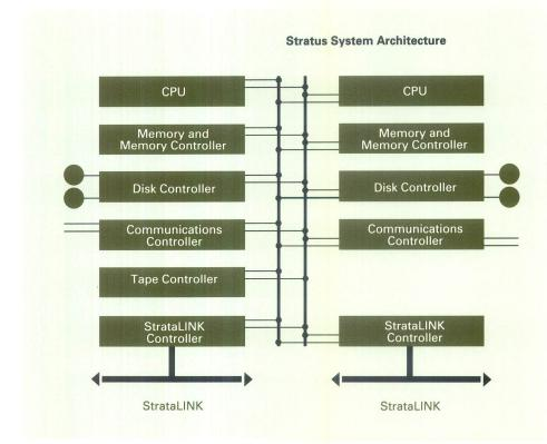
In a Stratus system, CPUs, memory, I/O controllers including disks and communications controllers, disks, power supplies, and buses are all duplicated to maintain processing should one component fail.
