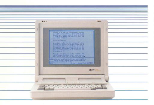
The Z-181 boasts perhaps the most advanced screen available in a laptop... display images are crisp, bold and bright. The Z-181 runs IBM PC/XT compatible software at up to 8 MHz and has an interface for a hard disk drive.
