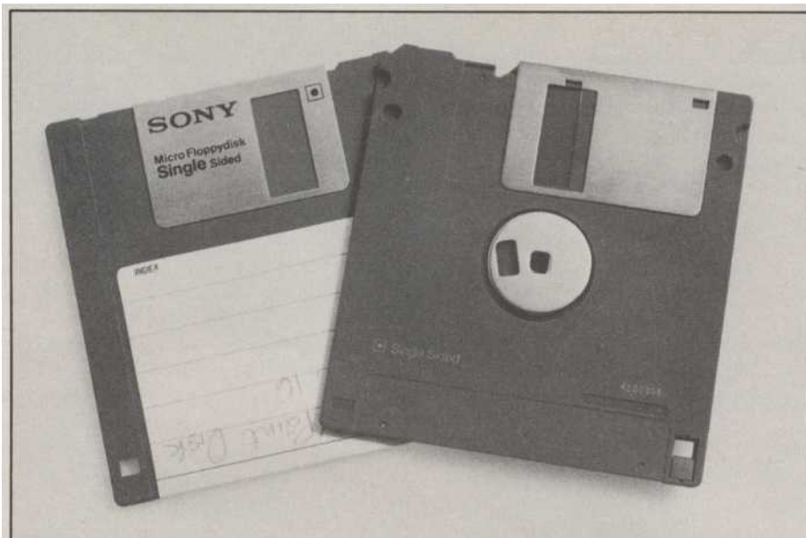
Photo 4: The Sony 3½-inch disk is encased in a rigid plastic housing, and the oval window through which the magnetic medium is accessed is protected by a metal shutter that slides out of the way when the disk is inserted in the drive. These factors help protect the disk from casual use.
