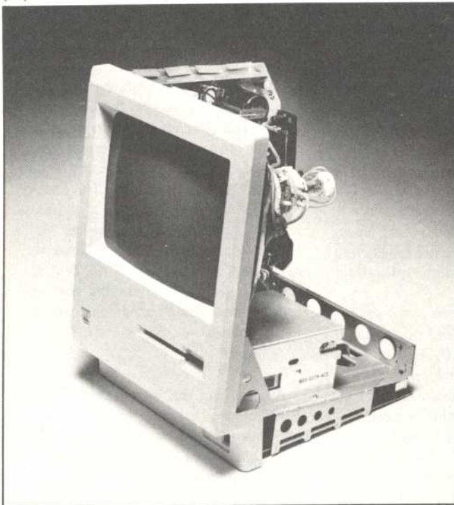
Photo 3: Inside the Macintosh computer. From the front (photo 3a), you can see the video display and the 3 1/2-inch disk drive. From the rear (photo 3b), you can see the two main circuit boards (right and bottom), the rear of the video-display tube, the 3 1/2-inch disk drive, and a row of connectors at the bottom of the unit. The connections go, from left to right, to the mouse, a second disk drive, two peripherals (these are two serial ports), and an external amplifier (for sound output).
