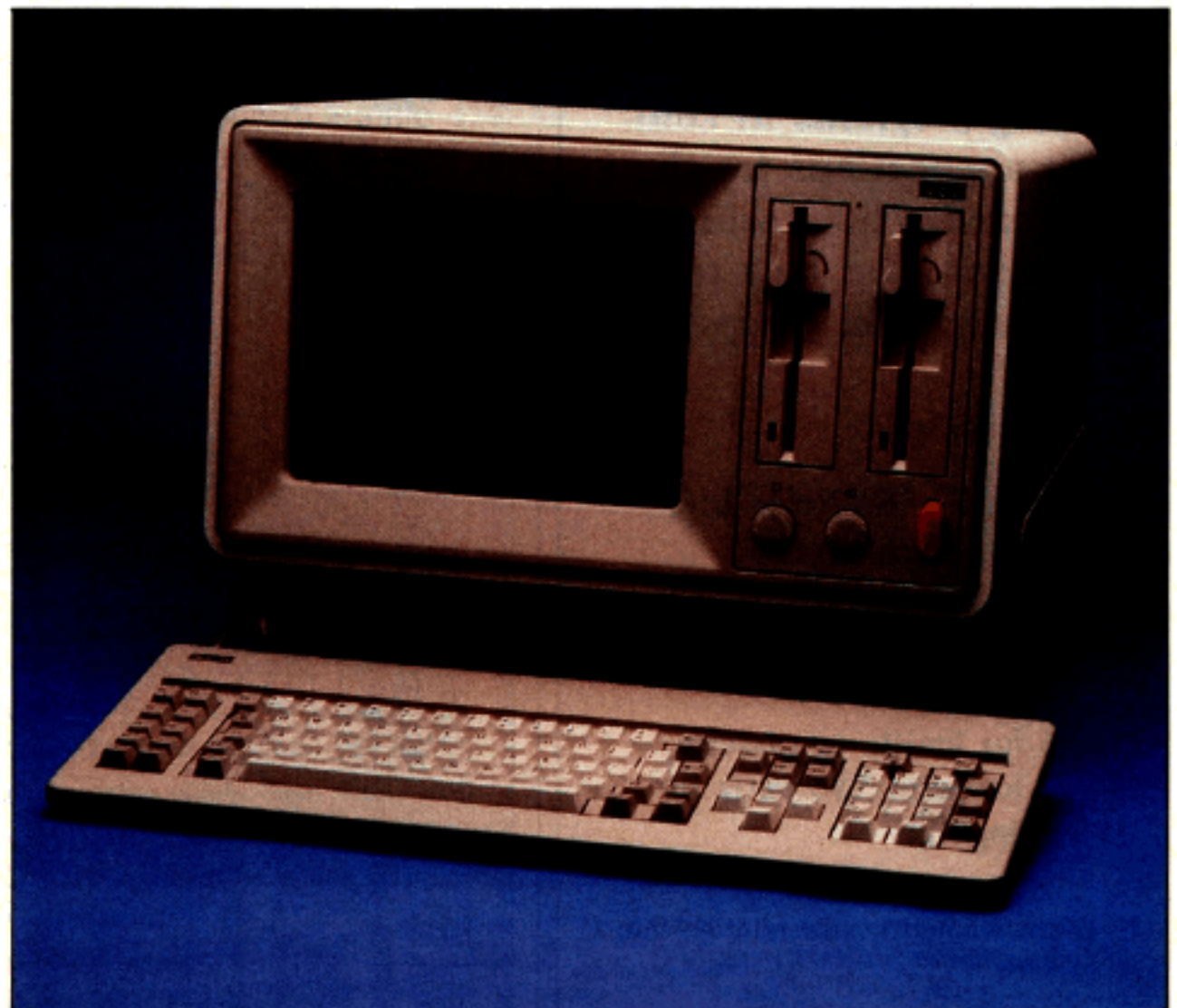
Photo 1: The NCR Model 4 with two vertical disk drives.
