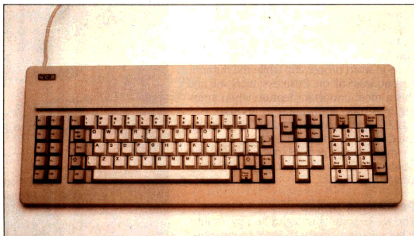
Photo 2: The keyboard, sold separately by NCR, is plug-compatible with the IBM PC and the Compaq Deskpro.
