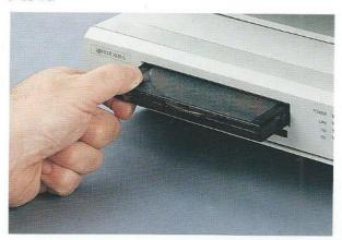
The XEN-S 240x provides 44 Mbytes of disk storage housed on an exchangeable media cartridge.
