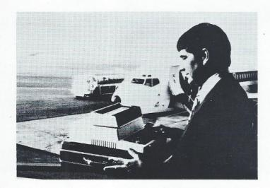
As a portable computer, the Athena I™'s size and weight is less than a portable typewriter's. An internal battery will operate the system for up to two hours or will retain the mass memory for up to six hours.
