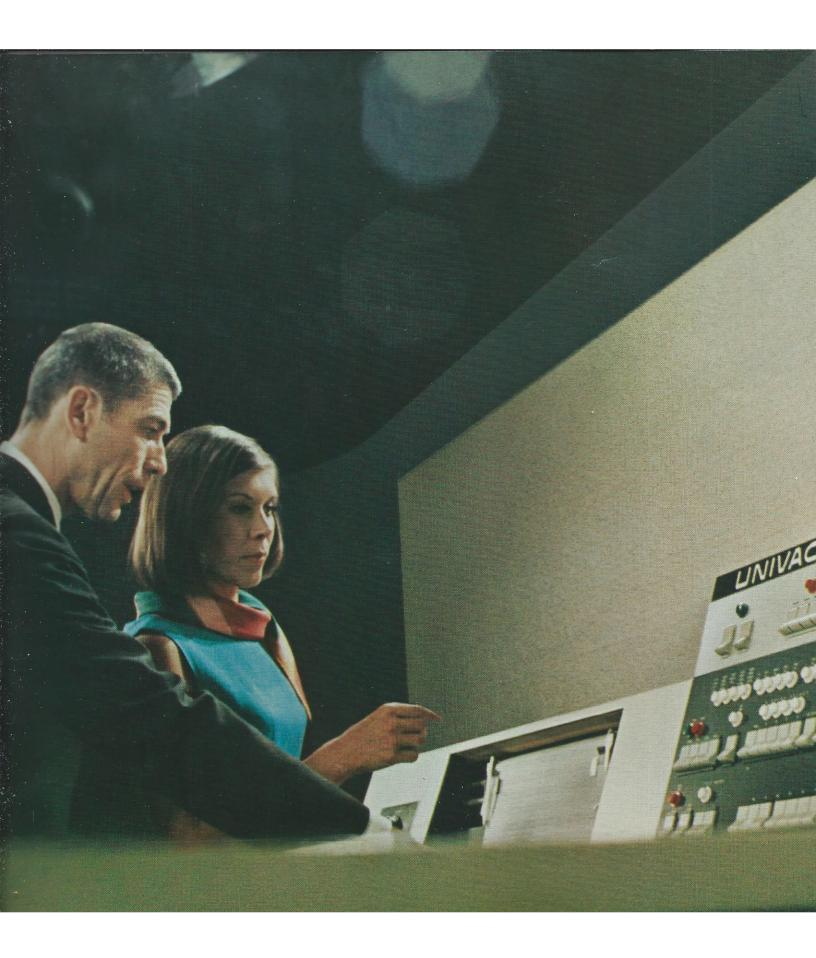
The UNIVAC 9200 is a compact, low priced system. It is internally programmed with punched card input-output and high speed printer. The computer is extremely fast, featuring a complete memory cycle time of 1.2 microseconds, and input-output time-shared with computation. Memory starts at 8,192 bytes and can be expanded to twice that size. (Each byte can hold two numeric or one alphabetical character.)
